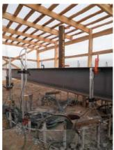
Pile head during bi-directional static load testing
